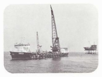
from the propulsion shaft and can be used to drive the alternators providing the power required by the 800-ton revolving crane. Power from the alternators is also tapped to drive the anchor winches, welding machines, pipe tensioners, gantry crane in the hold, and other electrical equipment. This arrangement enables one main engine to be used for propulsion purposes while the other drives an alternator should this power split become desirable.
