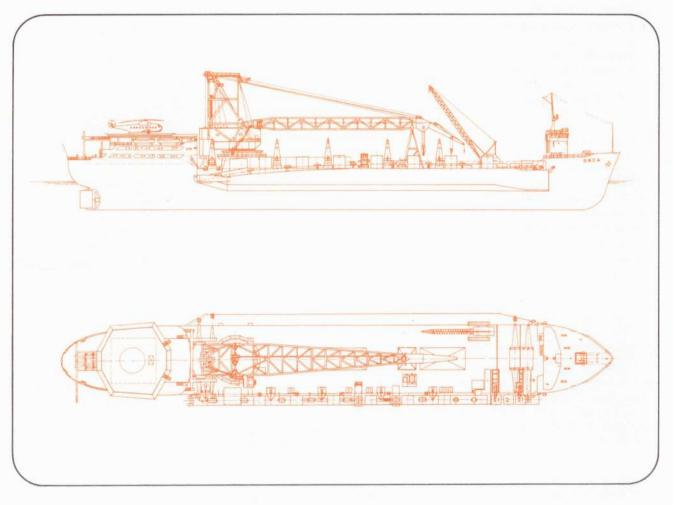
Late in May 1973, the multipurpose self-propelled workship Orca, operated by Netherlands Offshore Company established a new record for the heaviest over-the-side lift by a revolving crane offshore. It lifted into place the two deck-section modules of Conoco/NCB's 49/17, 8-pile production platform in the South Viking field off the U.K. One deck section weighed 800 tons, the other 750 tons.
