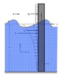
Figure 4: Wave loading on typical jack-up drill platform leg [5]
